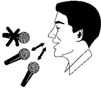
Illustration: Ideally, a handheld microphone should be positioned six to twelve inches from the user’s mouth, at an angle of 45 degrees or less. This usually avoids air currents that result in “popping” sounds when the consonants “P” or “T” are pronounced.
